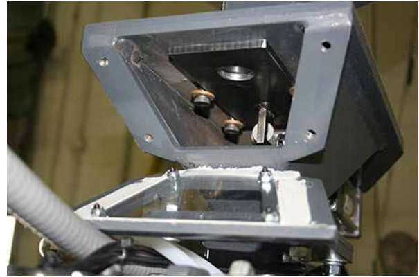
Orifice-based slide gate metering device (window guard removed for photo)
