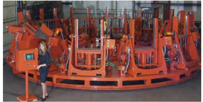
HALL 12 Station Rotary Table with RT2 Casting Machines (w/o molds installed)
