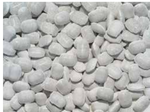
Figure 5: Illustration of Na-BF sodium oxide-based electric furnace and pressure pour flux.
