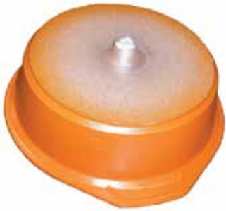
High End Casserole w/Riser Cast on a HALL RT3 Machine
