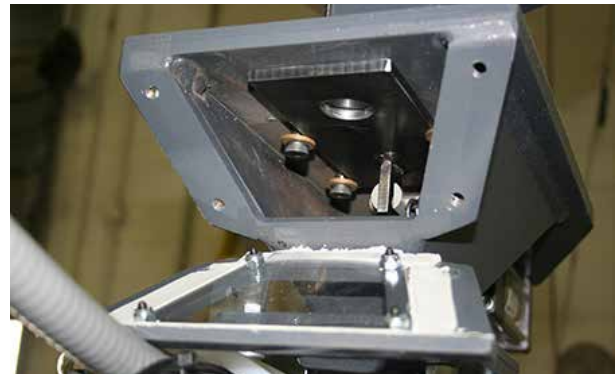
Orifice-based slide gate metering device (window guard removed for photo)
