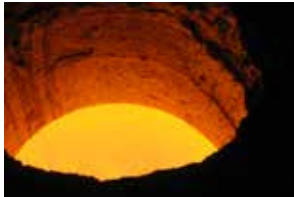
Figure 6: 184th Heat Furnace A treated with NaBF flux
