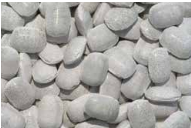
Figure 5: Illustration of Na-BF sodium oxide-based electric furnace and pressure pour flux.
