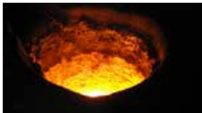
Figure 8a and 8b: Heat 260 on Furnace B - Untreated, taken out of service to be relined
