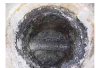
Figure 12a and 12b: 1 ton Tundish Ladle after treatment with the NaBF flux
