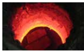
Figure 10a and 10b: 373rd Heat - Furnace A treated with the NaBF flux
