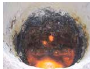
Figure 11a and 11b - 1 ton Tundish Ladle before treatment with a NaBF
