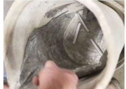
This skin contains oxides and should be removed prior to filling the ladle.
