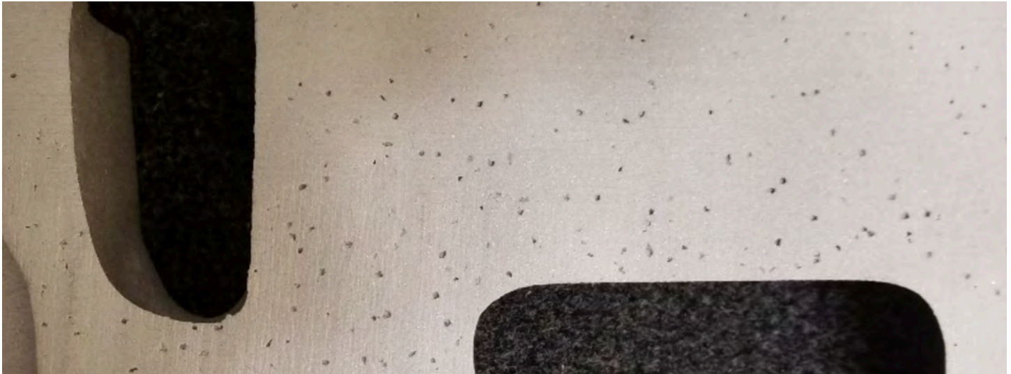
This part displays “Hydrogen Porosity”. Its cause is completely different than the other 5 types of porosity. Understanding the differences is key to solving the problem.
