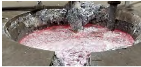
The dross build-up on this melt furnace will certainly add to the foundry scrap rate.
