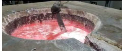
The same melt furnace after cleaning will result in less casting scrap.
