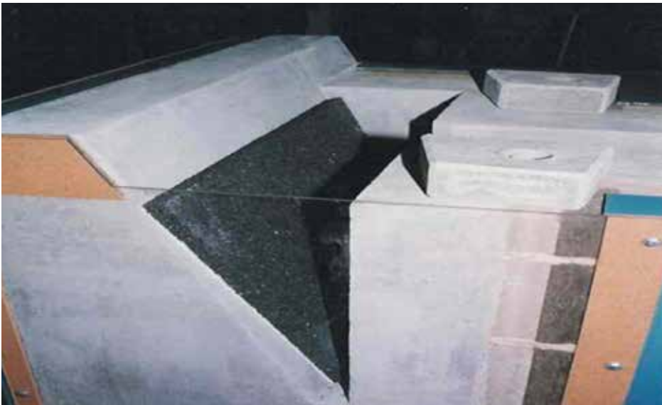
Figure 2: In-line 8 grit filter for a machine side melter or launder system
