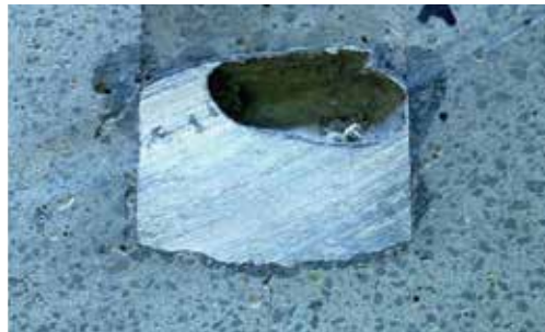
Figure 3. Corrosion test displaying non-wetting property of Blasch Nitron™
